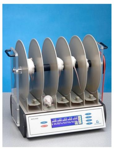
Most Huntington's disease model animals don't develop the involuntary movements that are seen in human patients. Tests like this spinning rod, called the 'Rotarod', are one way of measuring movement problems in rodents.
